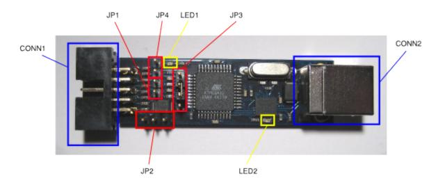
Figure 2.1: The USBprog device (version 3.0) with all connectors, jumpers and LEDs
